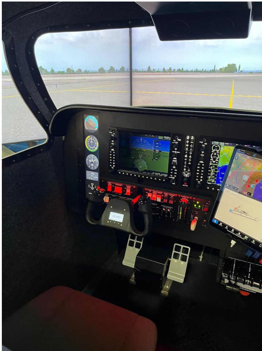
Sample of a typical LCD TV screen curved screen layout (standard FNPT II cockpit shown here)
